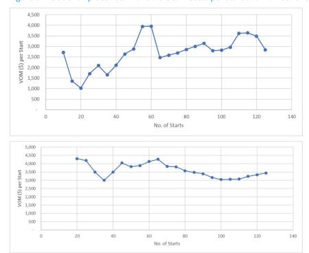
Figure 6: Relationship between Variable O&M Costs per start and number of starts – Pinjar Units
