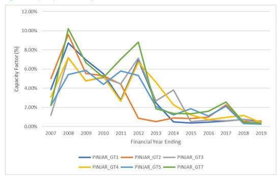
Figure 1: Capacity factor of Pinjar Units
