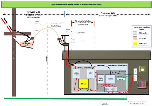
Figure 2 Typical Overhead Installation
