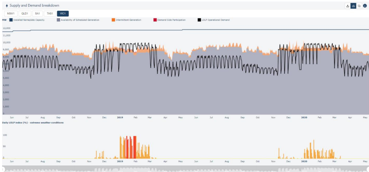
Figure 9Figure 14 Supply demand breakdown and maintenance period overview from LOLP run (User to select region and year)
