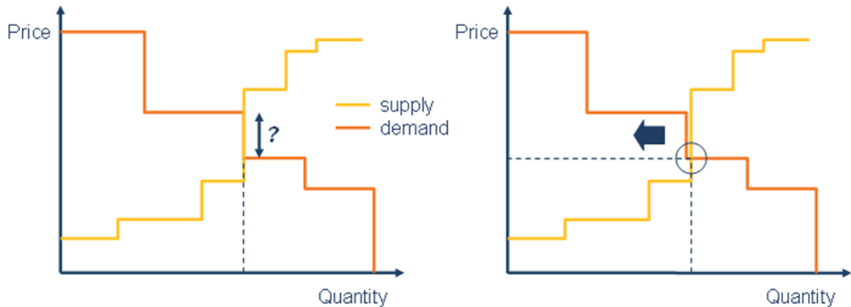
Figure 17 Market-clearing price ambiguity is resolved by subtracting a small value from the total demand
