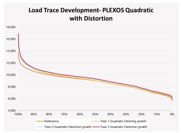
There is no one-size-fits-all set of parameters for these two quadratic parameters. A manual tuning process is undertaken during the demand growth process to ensure the parameters yield appropriate results for each region, and across simulation years.
