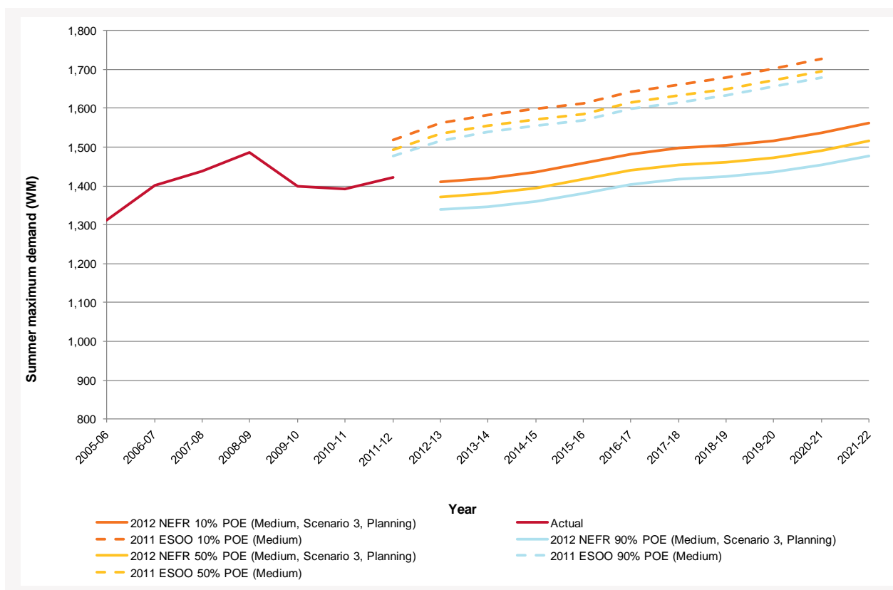
Figure 7-6 — Comparison of the 2012 NEFR and 2011 ESOO summer maximum demand forecasts for Tasmania
