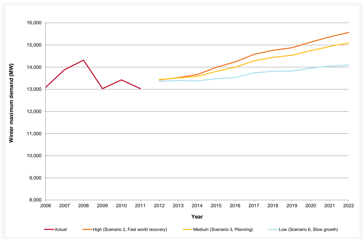
Figure 4-7 — Winter 50% POE maximum demand forecasts for New South Wales (including the ACT)
