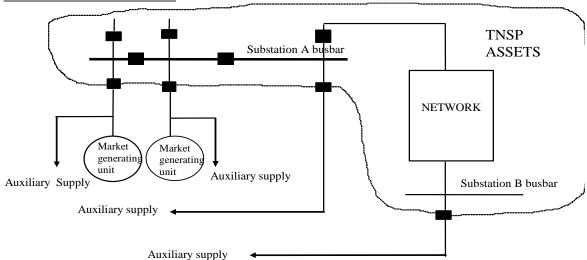
In all cases above, auxiliary supply for the *market generating unit* is taken from physically separated *connection points*, either at the same substation, or another point in the *network*, or a combination of local and remote points.
