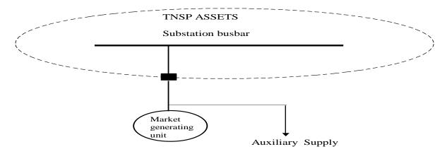
In this situation, the *Generator* is taking its auxiliary supply before the *transmission system*. Net consumption through this *connection point* would only be likely when the *generating system* is out of service, and only used to power the *generating system* at those times. In this case, the *Generator* is not required to register as a *Customer*. All purchases under this situation would be covered by clause 2.2.4(d) of the *Rules*.
