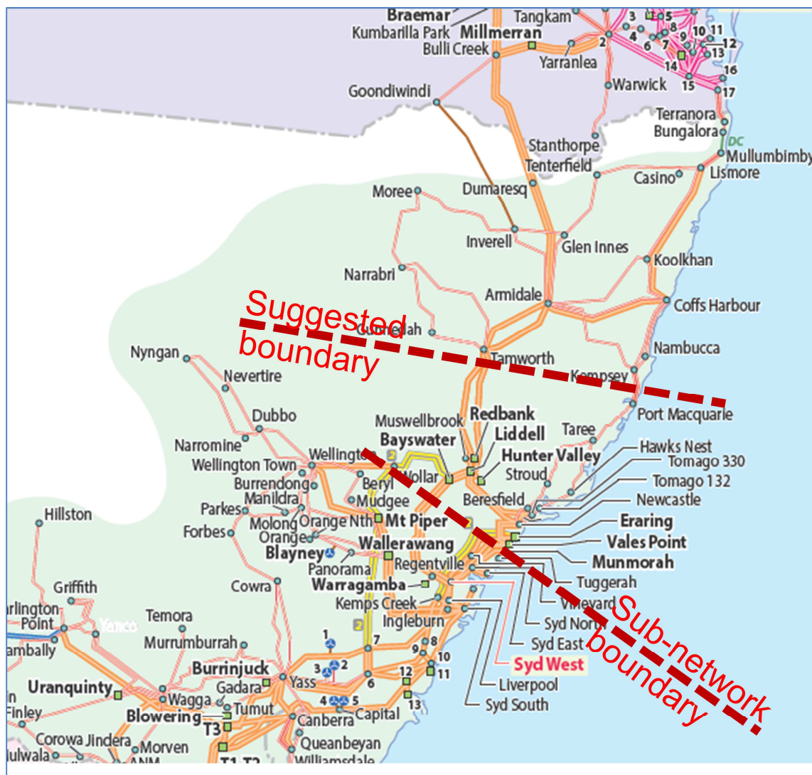
Figure 6: New South Wales transmission break point
