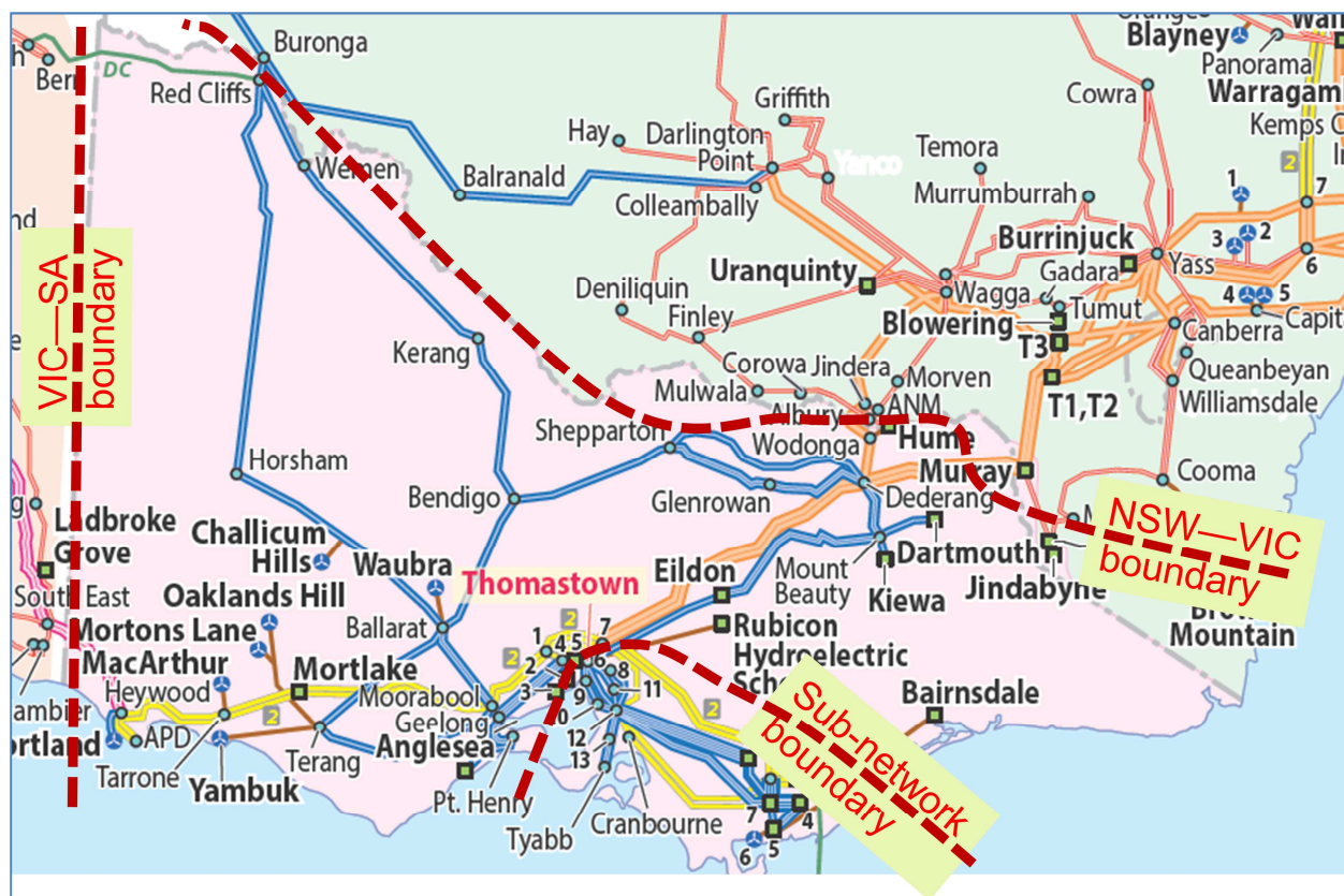
Figure 7: Victoria transmission break points
