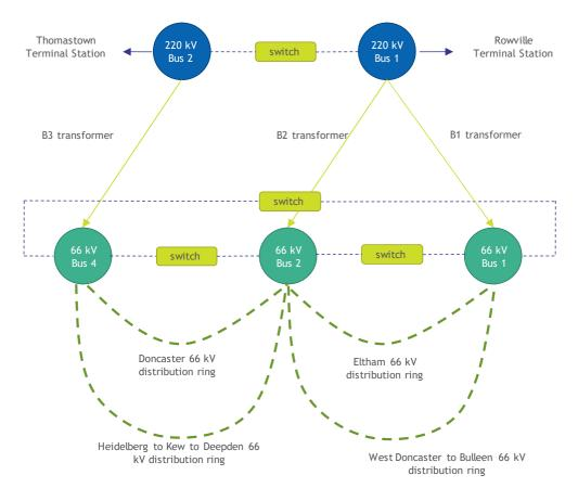
Figure 4 - Representative diagram for TSTS
