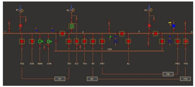
Figure 5 - BLTS 66 kV feeder arrangement and circuit breakers that need to be replaced
