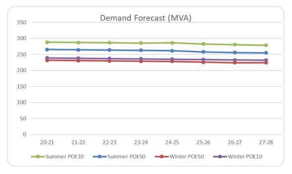
Figure 2 - Demand forecasts for BLTS 66 kV network
