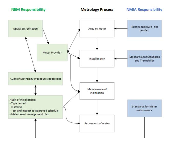
Note: The Act does not require meters to be verified when they are purchased. This is often common practice, but all that the Act requires is that meters must be verified before being used for trade (probably equivalent to installation for an electricity meter).
