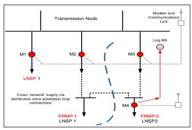
Transmission network connection point(s) feeding different  $\frac{LR - or}{LNSP}$  areas. The above configuration illustrates:
