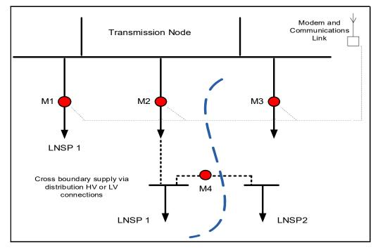
*Transmission network connection point(s)* feeding different LNSP areas. The above configuration illustrates:
