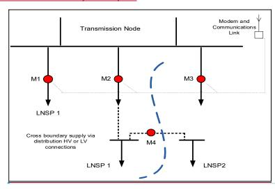
Transmission network connection point(s) feeding different LNSP areas. The above configuration illustrates:
