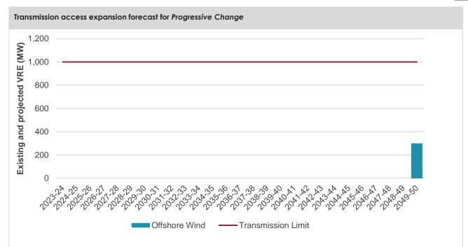
Note: There is no projected VRE in *Step Change* scenario. Therefore, no transmission expansion occurs in this REZ for the *Step Change* scenario to facilitate VRE connection in this zone.
