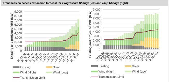
Note: Q3 forecast shows results for the NQ1 group constraint augmentation.
