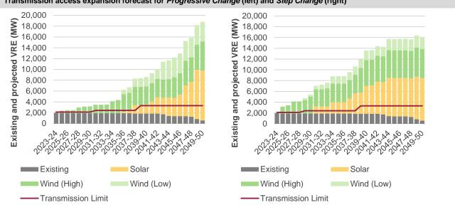
Note: Q6 forecast shows results for the NQ3 group constraint augmentation, including projected VRE for all REZs north of the NQ3; this includes Q1, Q2, Q3, Q4, Q5 and Q6. The transmission limit is modelled using the CNQ-SQ flowpath limit as opposed to a static number.
