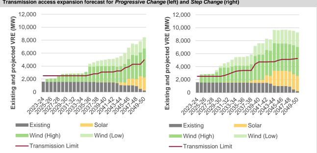
Note: Q4 forecast shows results for the NQ2 group constraint augmentation, which includes VRE projections for Q1, Q2, Q3, Q4 and Q5.
