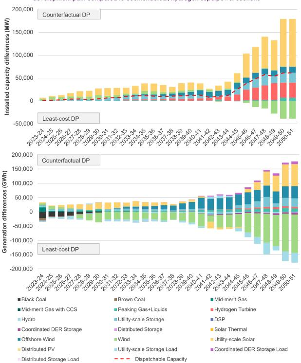
Figure 30 Forecast capacity developments (top) and generation (bottom) to 2050-51 for least-cost development path compared to counterfactual, Hydrogen Superpower scenario
