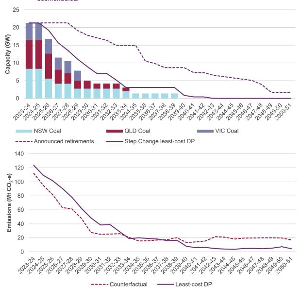
Figure 11 Forecast coal retirements (top) and emissions trajectory (bottom) to 2050-51, Step Change counterfactual
