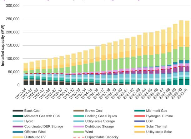
Figure 22 Forecast NEM generation capacity to 2050-51, Progressive Change scenario counterfactual
