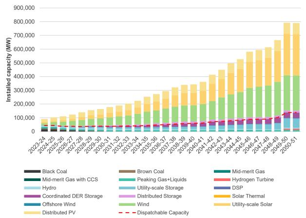
Figure 24 Forecast NEM generation capacity to 2050-51, Hydrogen Superpower scenario
