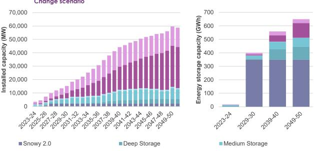
Figure 1 NEM storage MW capacity (left) and energy storage capacity (right) in the least-cost DP under Step Change scenario
