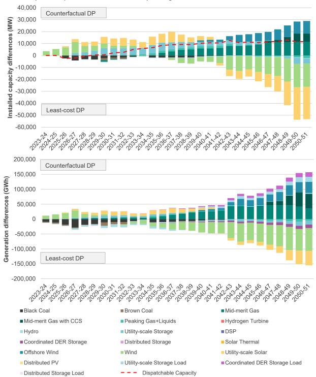
Figure 13 Forecast capacity developments (top) and generation (bottom) to 2050 for least-cost development path compared to counterfactual, Step Change scenario
