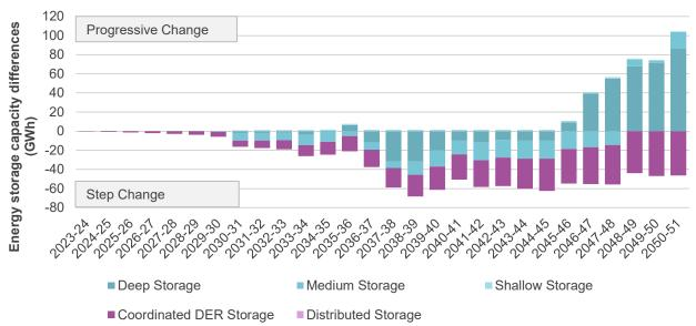
Figure 20 Comparison of energy storage capacity between Step change and Net Zero scenarios
