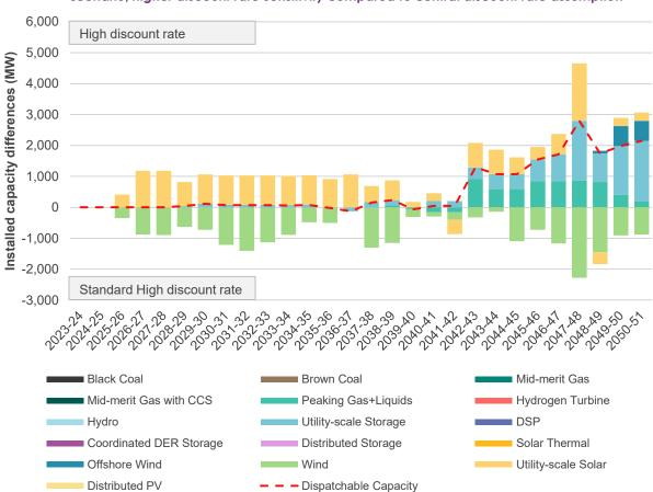
Figure 38 Forecast NEM generation capacity to 2050-51 for the least-cost DP in the Progressive Change scenario, higher discount rate sensitivity compared to central discount rate assumption
