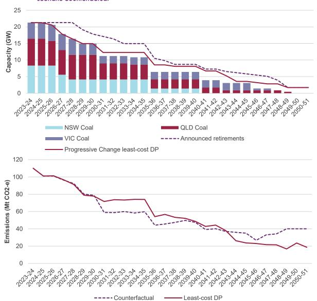
Figure 21 Forecast coal retirements (top) and emissions trajectory (bottom) to 2050, Progressive Change scenario counterfactual
