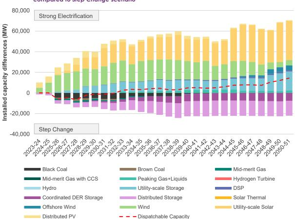
Figure 39 Forecast capacity developments to 2050-51 for least-cost DP of Strong Electrification sensitivity compared to Step Change scenario
