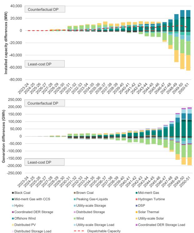
Figure 23 Forecast capacity developments (top) and generation (bottom) to 2050-51 for least-cost development path compared to counterfactual, *Progressive Change* scenario
