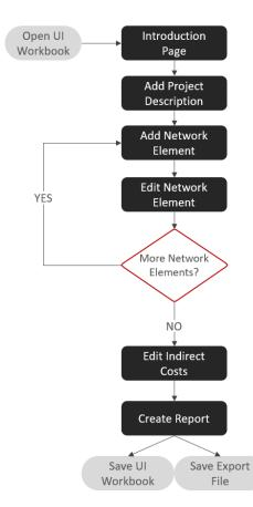
The stages within the black boxes of the cost estimation tool flowchart require user interaction. The following section will provide detailed user instructions for each stage to generate a project cost estimate using the cost estimation tool.
