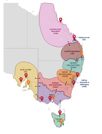
Figure 16 Electrolyser locations and their connections to electricity nodes
