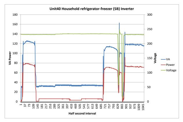
Unit:Unit41Sector:HouseholdProduct:refrigerator-freezer (5B)Motor type:InverterControl:ElectronicBrand:ElectroluxModel:EBE4507SA
