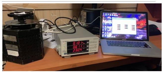
Figure 1: Equipment used to measure electrical characteristics at low voltage
