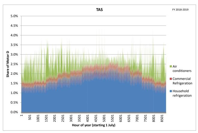
Figure 95: Hourly Motor D load for all covered loads in Tasmania, 2018-19
