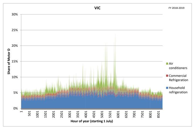
Figure 96: Hourly Motor D load for all covered loads in Victoria, 2018-19
