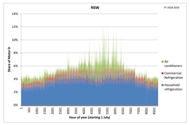
Figure 93: Hourly Motor D load for all covered loads in NSW and ACT, 2018-19 (2)
