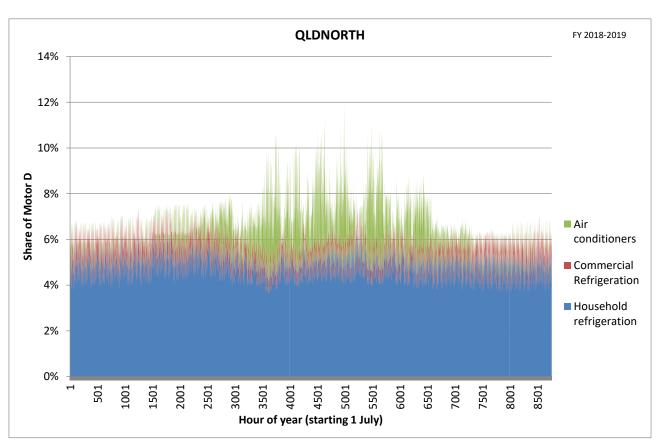
Figure 99: Hourly Motor D load for all covered loads in Queensland North, 2018-19
