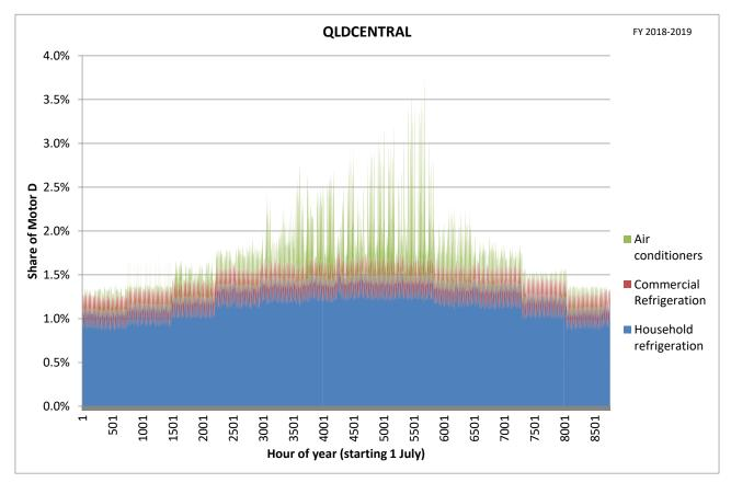
Figure 98: Hourly Motor D load for all covered loads in Queensland Central, 2018-19
