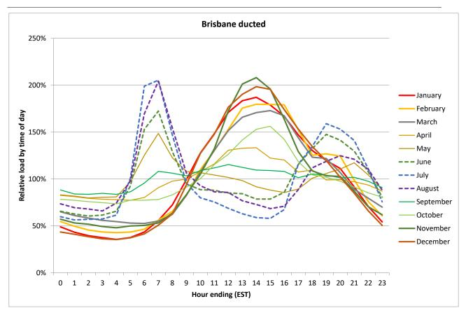
Figure 55: Relative time-of-day profile for ducted air conditioners, Brisbane
