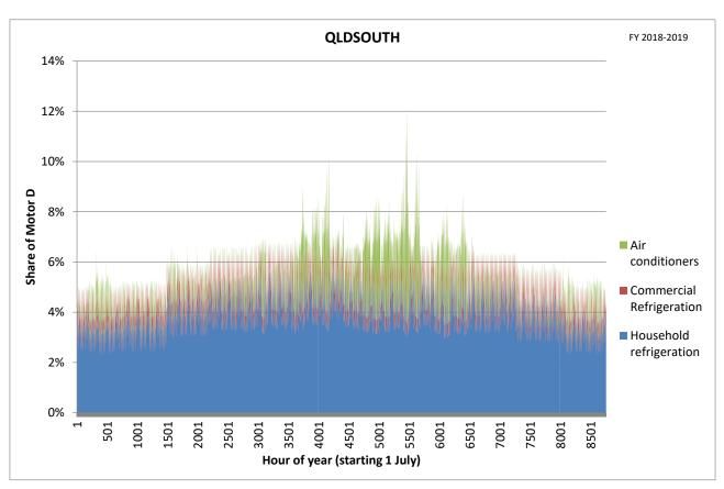
Figure 97: Hourly Motor D load for all covered loads in Queensland South, 2018-19
