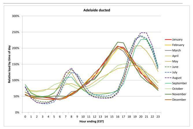
Figure 57: Relative time-of-day profile for ducted air conditioners, Adelaide
