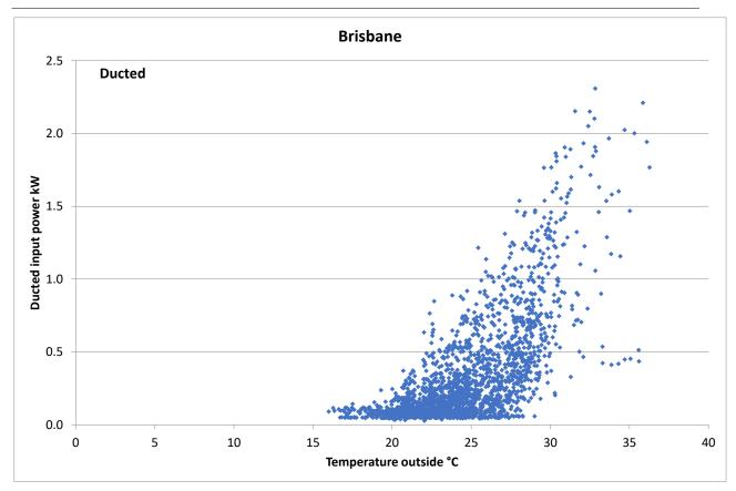
Figure 48: Hourly outdoor temperature vs ducted power data for Brisbane: Jan, Feb and Dec 2012
