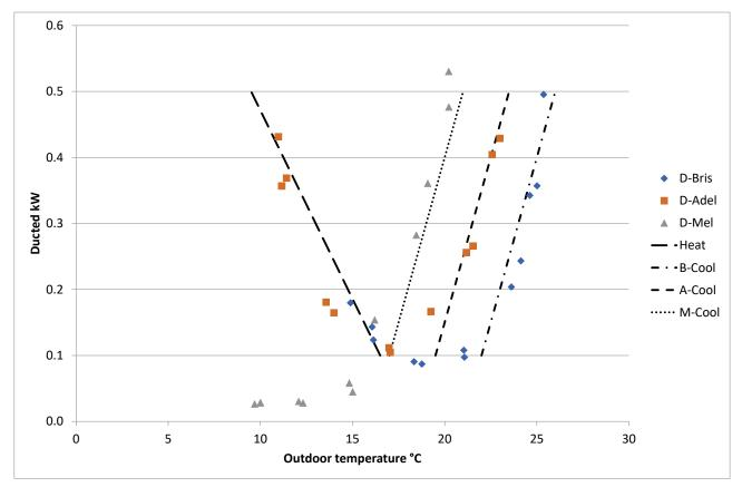
Figure 53: Average monthly ducted air conditioner by outdoor temperature
