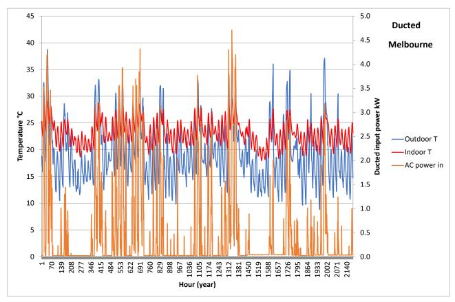
Figure 46: Hourly temperature and ducted power data for Melbourne: Jan, Feb and Dec 2012
