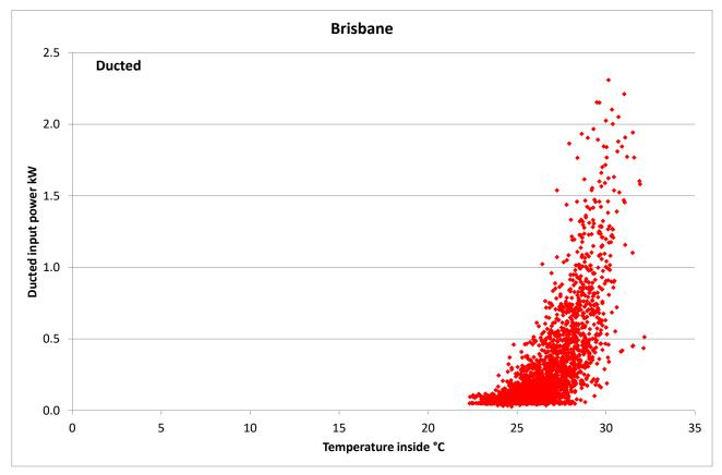
Figure 47: Hourly indoor temperature vs ducted power data for Brisbane: Jan, Feb and Dec 2012
