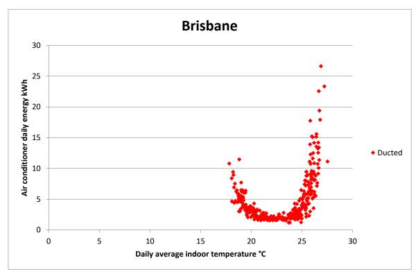
Figure 49: Daily average indoor temperature versus ducted air conditioner energy: Brisbane, 2012
