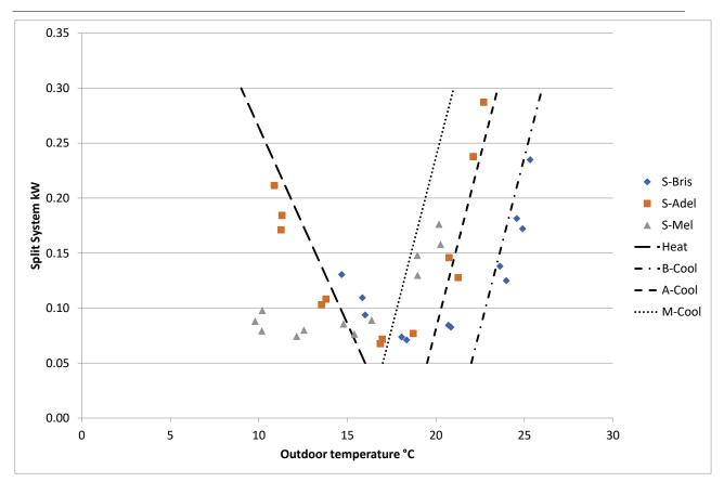
Figure 54: Average monthly ducted air conditioner by outdoor temperature
