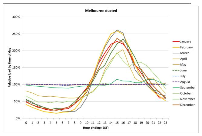
Figure 59: Relative time-of-day profile for ducted air conditioners, Melbourne
