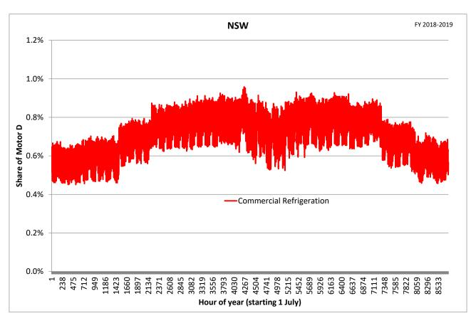
Figure 91: Hourly Motor D load for commercial refrigeration in NSW and ACT, 2018-19
