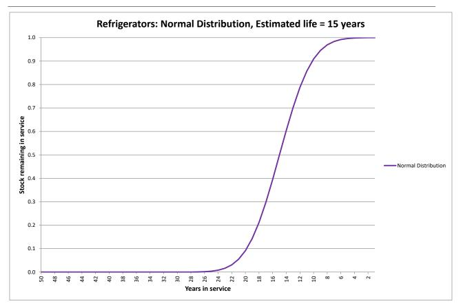
Figure 68: Retirement function (stock remaining) for refrigerator stock model
