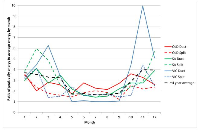
Figure 52: Ratio peak daily energy to average energy by equipment type and city: 2012 Notes: 4 year average shown is across all equipment types and years 2012 to 2015 inclusive.
