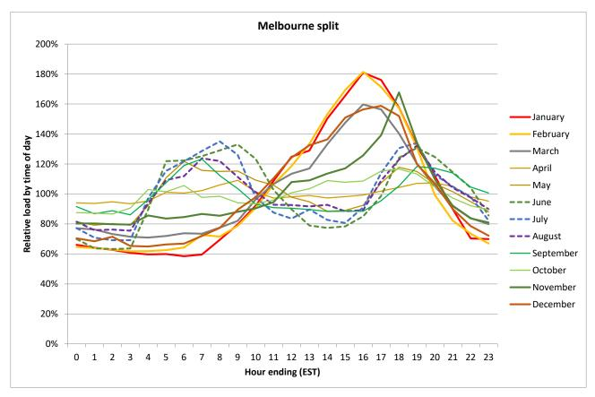
Figure 60: Relative time-of-day profile for split air conditioners, Melbourne
