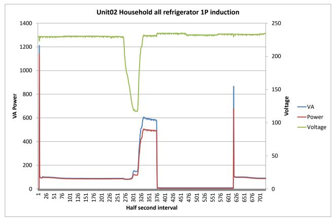
Figure 20: Example of low voltage stall data for a household refrigerator
