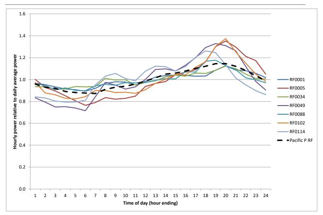
Figure 80: Normalised time-of-day for a selection of refrigerators
