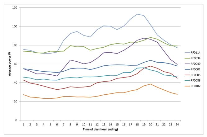
Figure 79: Time-of-day average power for seven refrigerators (Harrington 2018)
