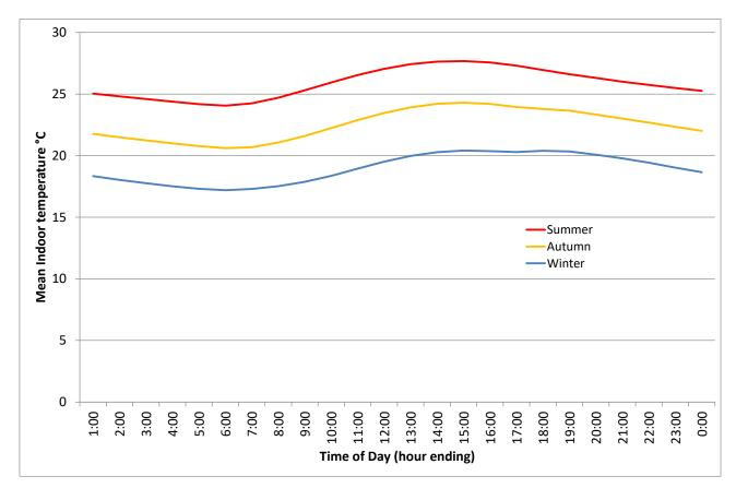
Figure 76: Seasonal indoor temperature profiles for houses in Brisbane (Harrington 2018)
