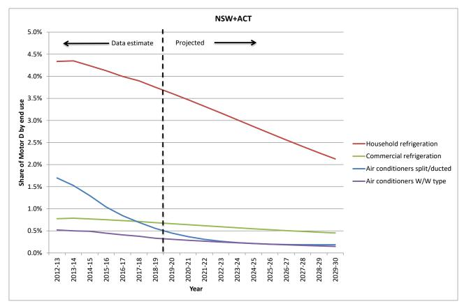
Figure 106: Projected share of Motor D of underlying system load by end use for NSW and ACT
