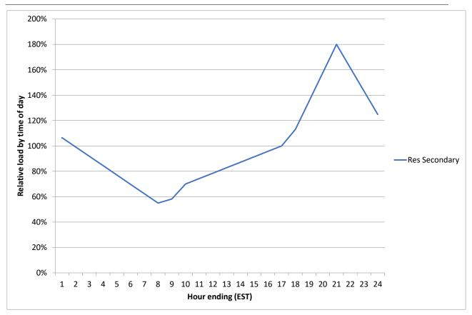
Figure 62: Generic air conditioner time-of-day load shapes – residential secondary air conditioners
