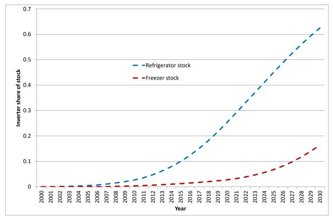
Figure 70: Stock share of inverter driven refrigerators and freezers in Australia
