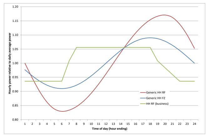
Figure 82: Generic load profiles for refrigerators and freezers
