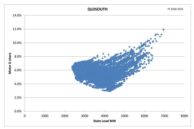
Figure 104: Motor D share versus underlying system load for Queensland South in 2018-2019
