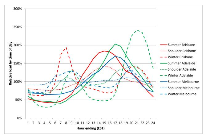
Figure 61: Generic air conditioner time-of-day load shapes - residential main air conditioners
