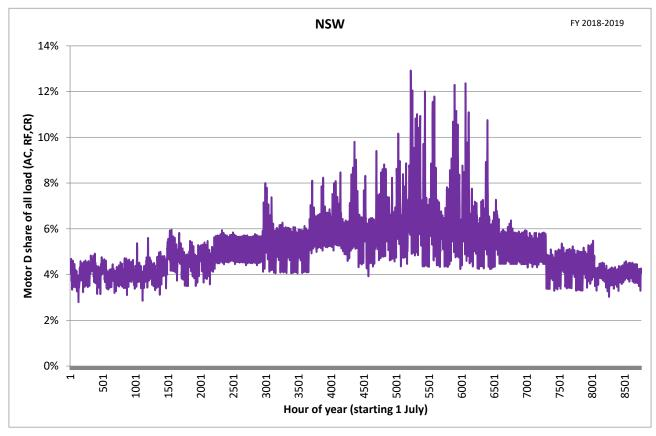
Figure 92: Hourly Motor D load for all covered loads in NSW and ACT, 2018-19 (1)
