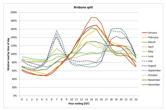
Figure 56: Relative time-of-day profile for split air conditioners, Brisbane
