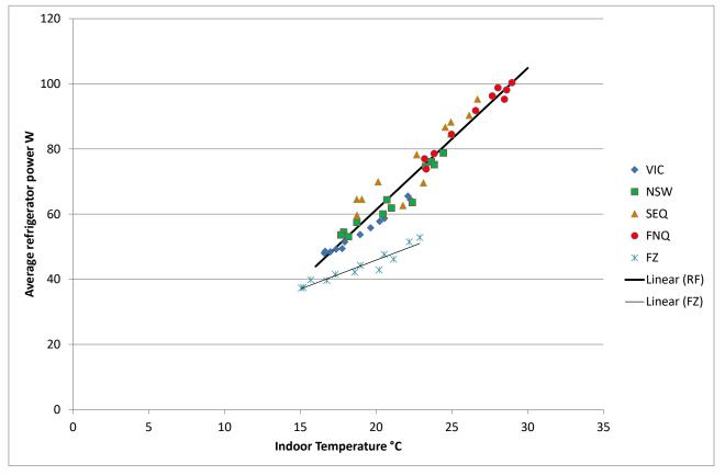
Figure 71: Model of power versus indoor temperature for household refrigerators and freezers
