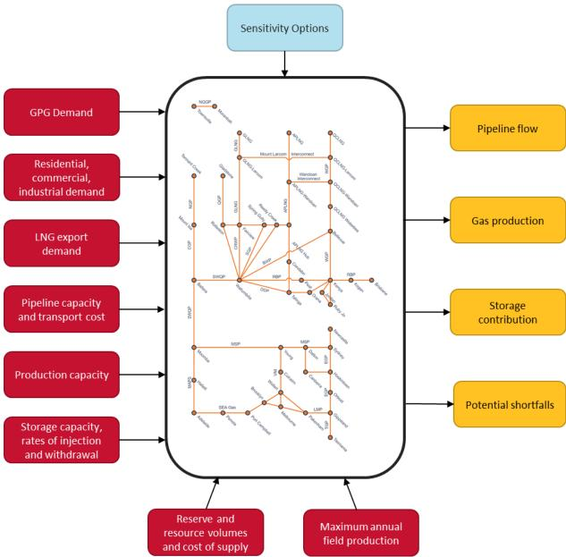
The eastern and south-eastern gas network is represented by a series of connected nodes. At each node, gas may be injected into or withdrawn from the network where production facilities and loads are connected respectively.
