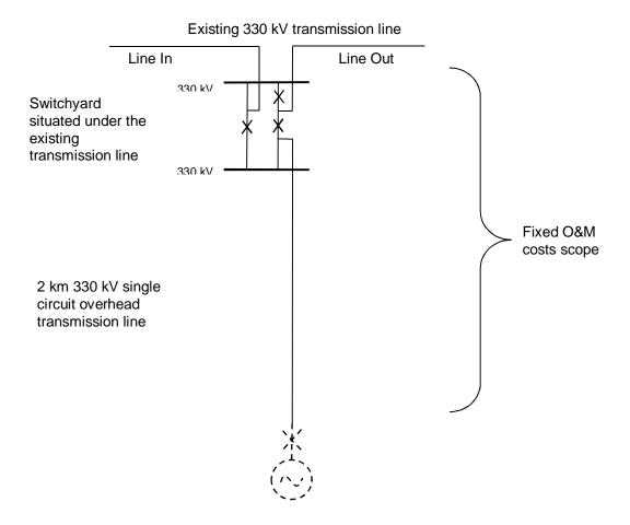
The new transmission line is assumed to be a single circuit 330 kV construction with 2 conductors per phase. The rating of the line has been selected to facilitate the transport of up to 200 MVA (at a power factor of 0.8, a 160 MW OCGT can export up to 200 MVA).
