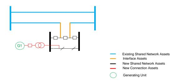
Figure 2: New Terminal Station (after commissioning) (Click to enlarge)
