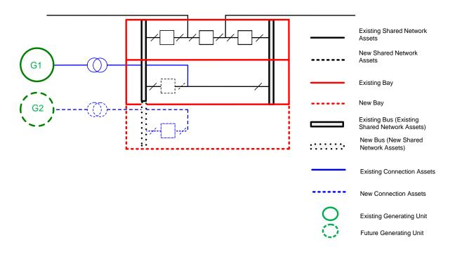
Figure 4: Connection to an Existing Sub-station (After Commissioning of Second Connection)
