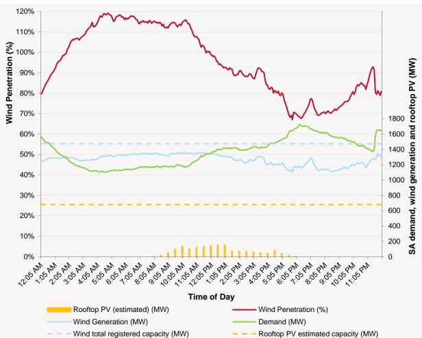
Figure 1 South Australian wind generation, demand, rooftop PV, and wind penetration for 22 May 2016
