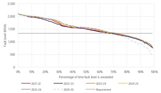
Figure 3 System strength outlook for Risdon under the traditional operations projections
