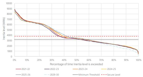
Figure 5 Inertia outlook for Tasmania under the traditional operations projection
