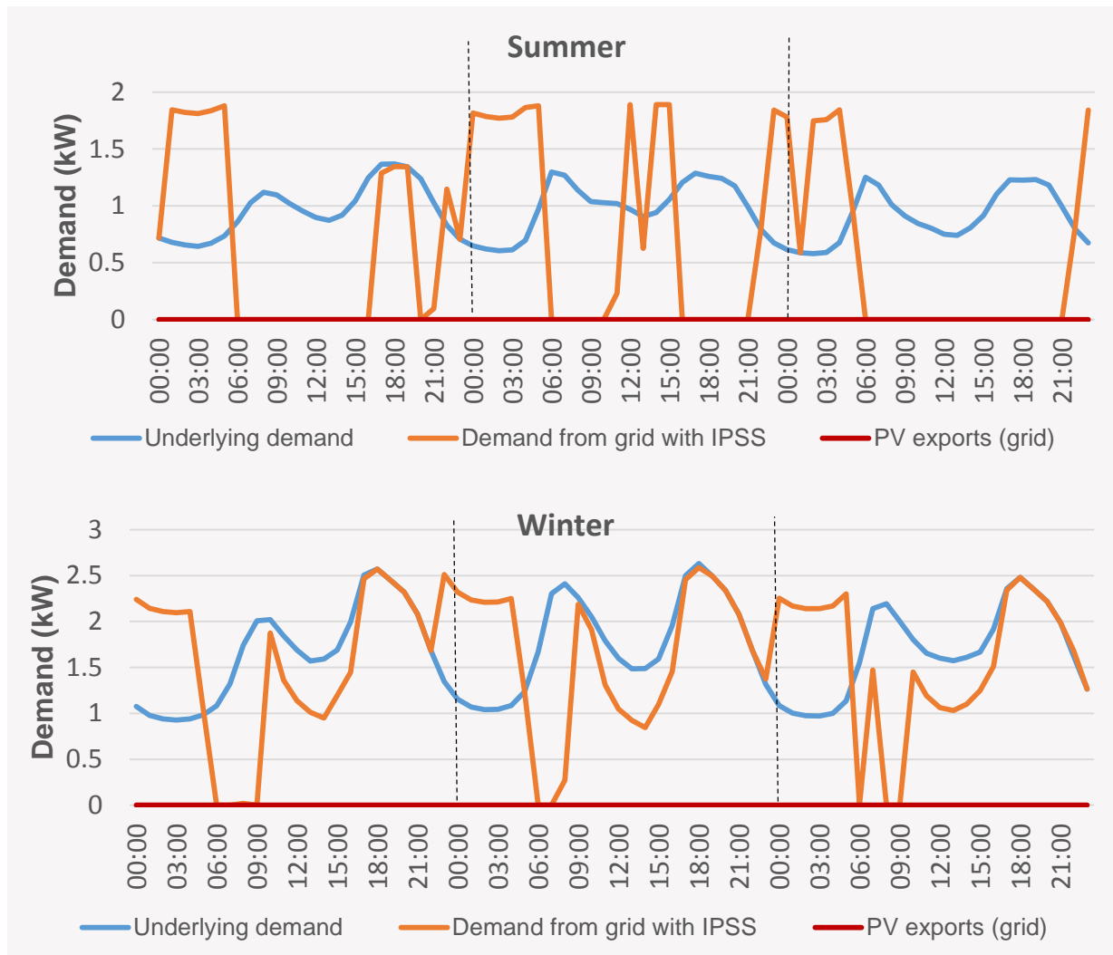
Figure 34 Forecast impact of IPSS on daily load profile of large consumer in Tasmania around times of regional maximum demand
