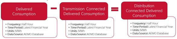
Transmission connected consumption was assumed to be business load, and was separated from the total demand to keep AEMO's meter data on the same basis as the AER's percentage splits.
