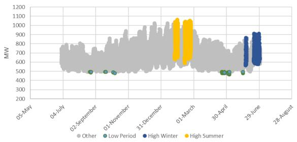
Scaling then commences. The demand, categorised into day-types, is scaled according to the ratios in Table 20. The ratios are calculated as *target / prepared trace* using the information from Table 19.
