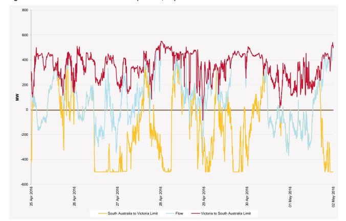
Figure 11 Interconnector limits in actual operation, Heywood Interconnector
