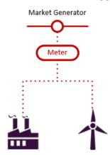
This scenario includes a scheduled generator and a semi-scheduled generator: one gas fired turbine and one wind farm. The wind farm requires an ECM, there would be separate dispatchable units each with a DUID and appropriate SCADA metering. A single GPS would
