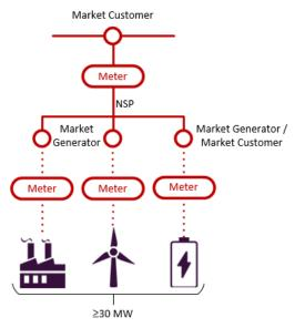
This scenario includes a semi-scheduled generating unit and two scheduled generating units: one wind farm, one gas fired turbine, and one battery that charges from the grid. The three systems are connected into a private network and operate independently of each other with individual registration, conformance cap for wind farm, GPS (which need to consider each other in the modelling), dispatch, SCADA and ECM for the wind farm.
