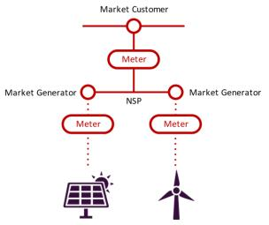
In the above scenario, the proponent has elected to establish two separate generating systems within an embedded network for business reasons. To meet rule requirements, the Embedded Network will need to be a registered Network. This requires a parent child metering arrangement to be established, for settlement purposes.
