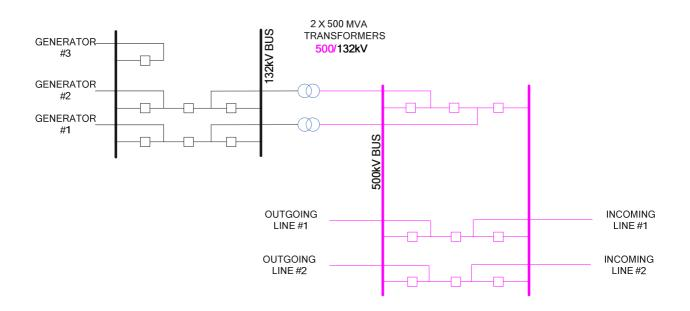
Figure 12: Stage 2 of 500/132 kV Hub for Connecting Generating Capacity in the Range of 500 MVA - 1,000 MVA
