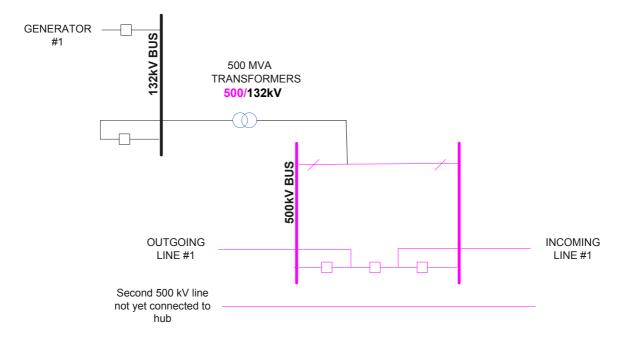
Figure 11: Stage 1 of 500/132 kV Hub for Connecting Generating Capacity in the Range of 0 MVA - 500 MVA
