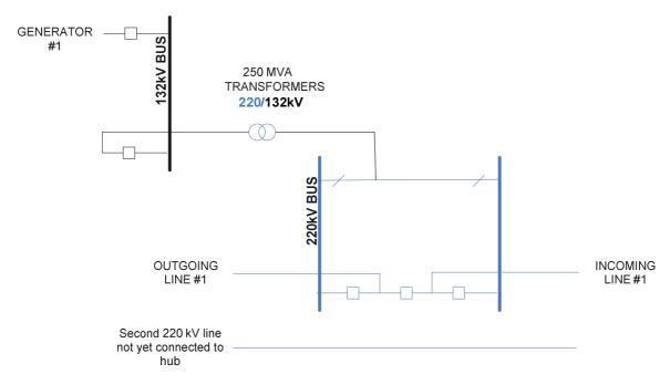
Figure 8: Stage 1 of 220/132 kV Hub to Connect Generation Capacity in the Range 0 MVA - 250 MVA
