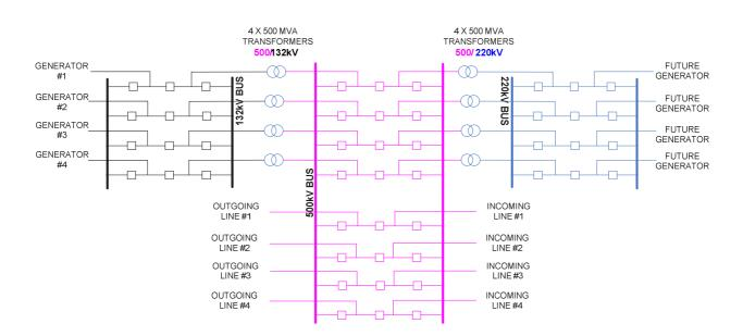
Figure 13: Stage 3 - Ultimate Layout of 500/220/132 kV Hub
