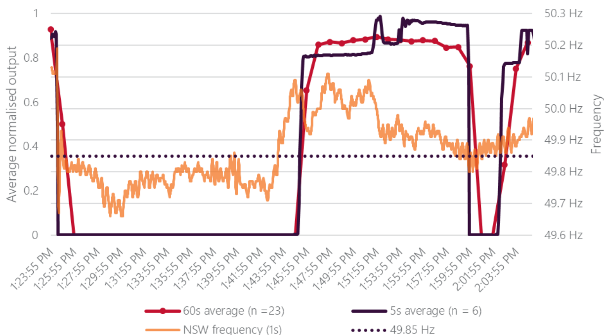
Figure 17 Average normalised output of distributed PV systems responding to frequency in NSW/QLD
