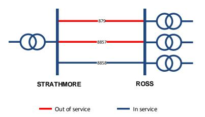
To manage power system security, AEMO invoked the constraint set Q-X\_SMRS\_A at 0645 hrs. This constraint set applies a limit of 260MW on the flow across the Ross cutset. This required an increase of generation in northern Queensland to reduce the cutset flow to the 260MW limit.
