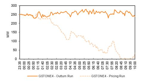
Figure 2 Dispatch of the Gladstone Power Station generating unit 4 under outturn and pricing runs
