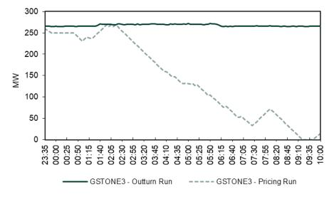
Figure 1 Dispatch of the Gladstone Power Station generating unit 3 under outturn and pricing runs
