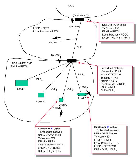
This example network shows how the associated connection points are to be registered within AEMO's system.
