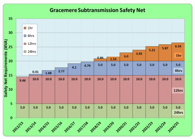
Figure 7 - Gracemere Subtransmission Safety Net Requirements
