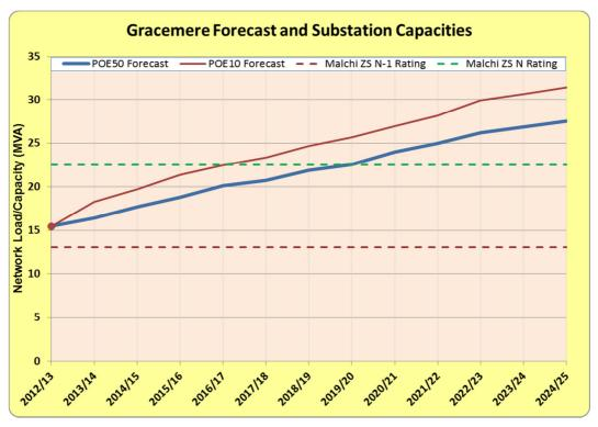
Figure 4 - Gracemere Forecast and Substation Capacity
