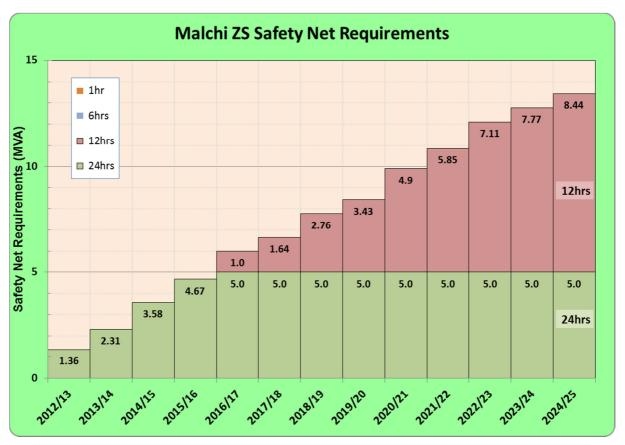
Figure 6 – Malchi Zone Substation Transformer Safety Net Requirements
